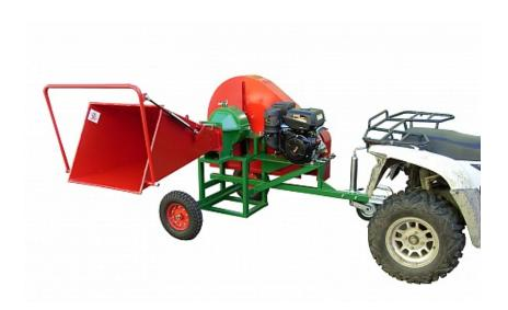
Machine equipment is designed for crushing branches, wood and wood waste, using two-way self-feeding cutting screw. The high performance of the machine is provided by the KOHLER petrol engine of 14Hp, which is by robust pulley geared to slow, to force. The machine has automatic feeder. The wood chipper takes branches with leaves, needles, branched, dry, wet, and takes also boards and beams.
