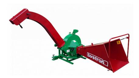
Machine equipment is designed for crushing branches, wood and wood waste, using two-way self-feeding cutting screw. The machine has automatic feeder and all functions are turned on mechanically. Required tractor power from 20 kW and more. The wood chipper takes branches with leaves, needles, branched, dry, wet, and takes also boards and beams.
