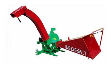
Machine equipment is designed for crushing branches, wood and wood waste, using two-way self-feeding cutting screw. The machine has automatic feeder and all functions are turned on mechanically. Required tractor power from 10 kW and more. The wood chipper takes branches with leaves, needles, branched, dry, wet, and takes also boards and beams.
