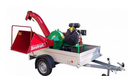
Machine equipment is designed for crushing branches, wood and wood waste, using two-way self-feeding cutting screw. The high performance of the machine is provided by the KOHLER ECH980 petrol engine of 38Hp(28,3kW). The machine has automatic feeder. The wood chipper takes branches with leaves, needles, branched, dry, wet, and takes also boards and beams.
