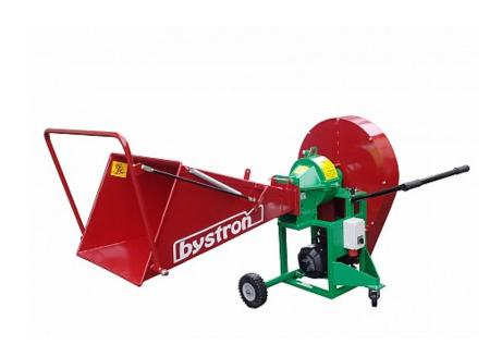
Machine equipment is designed for crushing branches, wood and wood waste, using two-way self-feeding cutting screw. The high performance of the machine is provided by the electric engine of 4KW, which is by robust pulley geared to slow, to force. The machine has automatic feeder. The wood chipper takes branches with leaves, needles, branched, dry, wet, and takes also boards and beams.
