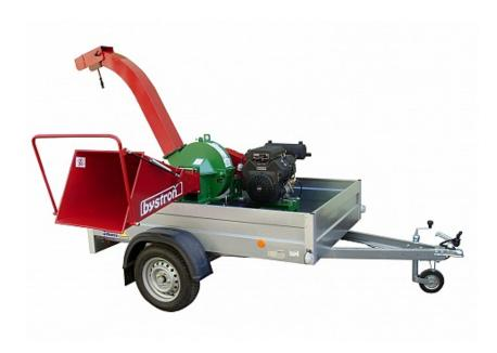
Machine equipment is designed for crushing branches, wood and wood waste, using two-way self-feeding cutting screw. The high performance of the machine is provided by the KOHLER petrol engine of 23.5Hp, which is by robust pulley geared to slow, to force. The machine has automatic feeder. The wood chipper takes branches with leaves, needles, branched, dry, wet, and takes also boards and beams.
