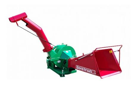
Machine equipment is designed for crushing branches, wood and wood waste, using two-way self-feeding cutting screw. The machine has automatic feeder and all functions are turned on mechanically. Required tractor power from 30 kW and more. The wood chipper takes branches with leaves, needles, branched, dry, wet, and takes also boards and beams.
