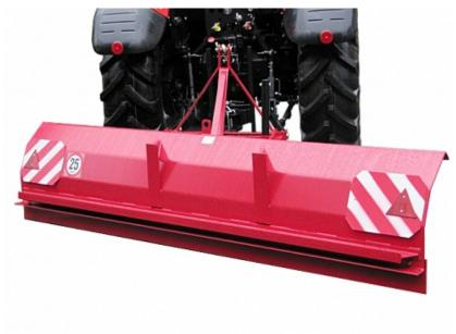
The machine is designed as a tractor attachment. The robust construction is welded and reinforced with thickened material, making it resistant to bending, cracking and other damage.
