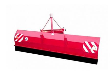
New type of blade designed for winter maintenance of roads and paved areas. The blade is used to remove fresh snow.
