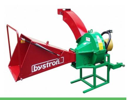
Machine equipment is designed for crushing branches, wood and wood waste, using two-way self-feeding cutting screw. The screw is supported by the support bearing, which prevents its offset. The machine has automatic feeder and all functions are turned on mechanically. Required tractor power from 20 kW and more. The wood chipper takes branches with leaves, needles, branched, dry, wet, and takes also boards and beams.
