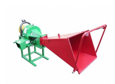
Machine equipment is designed for crushing branches, wood and wood waste, using two-way self-feeding cutting screw. The screw is supported by the support bearing, which prevents its offset. The machine has automatic feeder and all functions are turned on mechanically. Required tractor power from 10 kW and more. The wood chipper takes branches with leaves, needles, branched, dry, wet, and takes also boards and beams.
