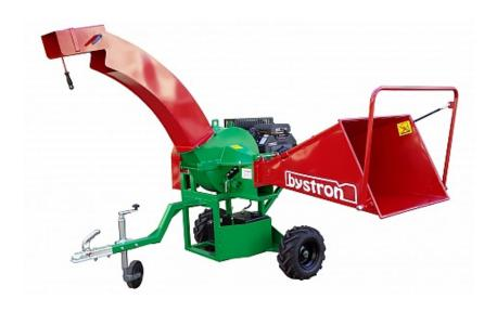
Machine equipment is designed for crushing branches, wood and wood waste, using two-way self-feeding cutting screw. The high performance of the machine is provided by the KOHLER petrol engine of 23.5Hp, which is by robust pulley geared to slow, to force. The machine has automatic feeder. The wood chipper takes branches with leaves, needles, branched, dry, wet, and takes also boards and beams.
