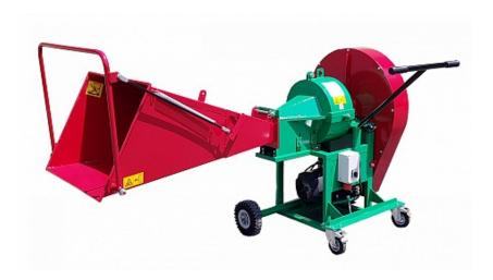
Machine equipment is designed for crushing branches, wood and wood waste, using two-way self-feeding cutting screw. The screw is supported by the support bearing, which prevents its offset. The high performance of the machine is provided by the electric engine of 4KW, which is by robust pulley geared to slow, to force. The machine has automatic feeder. The wood chipper takes branches with leaves, needles, branched, dry, wet, and takes also boards and beams.
