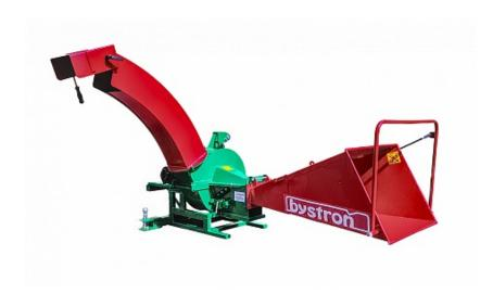
Machine equipment is designed for crushing branches, wood and wood waste, using two-way self-feeding cutting screw. The machine has automatic feeder and all functions are turned on mechanically. Required tractor power from 20 kW and more. The wood block chipper takes branches with leaves, needles, branched, dry, wet, and takes also boards and beams.
